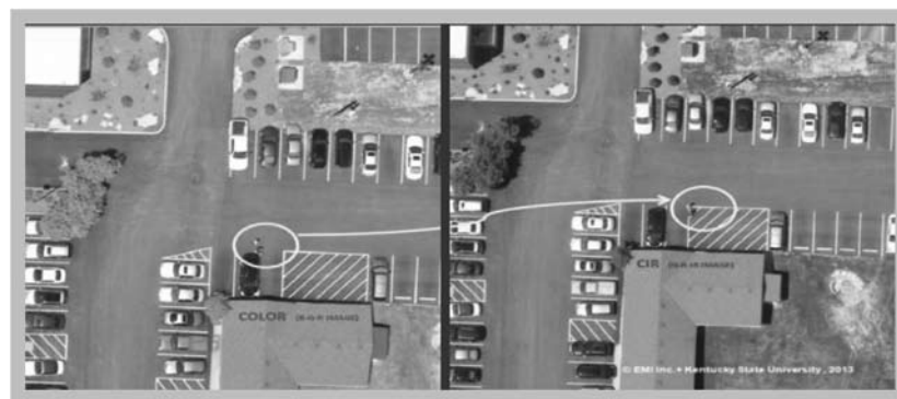
Figure 1: Sample 5-cm Resolution Orthoimagery of Bernheim Arboretum & Research Forest; Left: True Color, Right: Color Infrared (Source: EMI + KySU)
